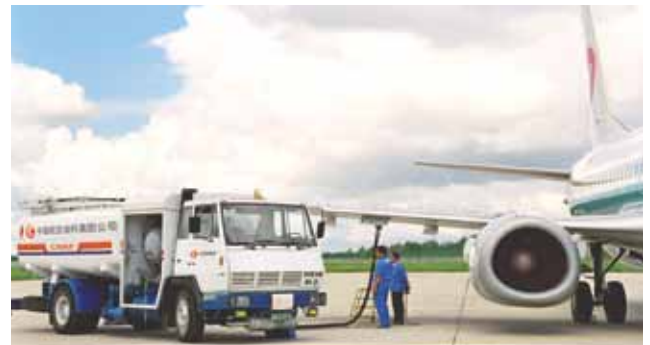
Into-plane refuelling operations of CNAF at a Chinese airport CNAF 在中国的航油加注业务
