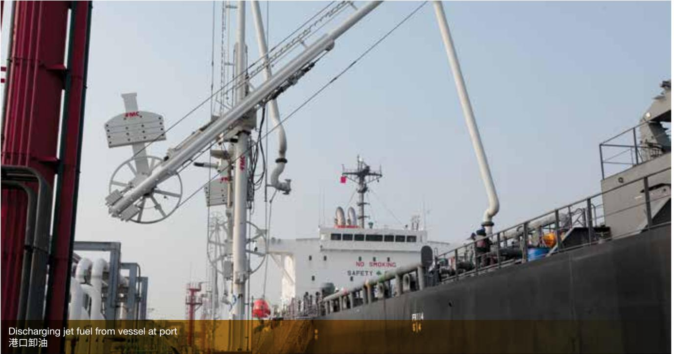
Discharging jet fuel from vessel at port
